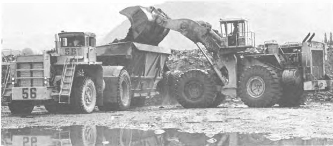
MICA PROJECT - 14 cubic yard loader filling 120 ton belly-dump unit. September 1969.
